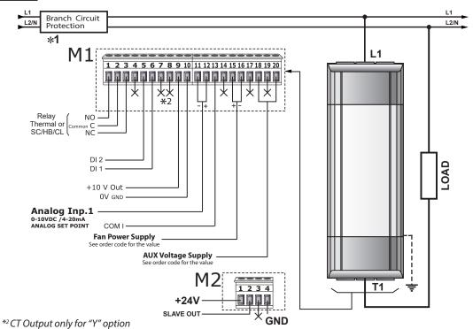
**Note:** Aux Voltage and Load Voltage must be synchronized
