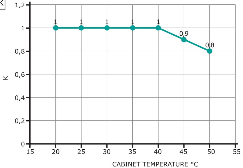
For higher cabinet temperature (more than 50°C) contact the producer of the unit
