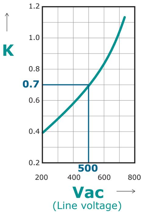
\*I<sup>2</sup>t are multiplied for K value in function of Vac, at 500V K is equal to 0,7 (ex:3100 X 0,7 = 2170). At 690Vac K is equal to 1.
