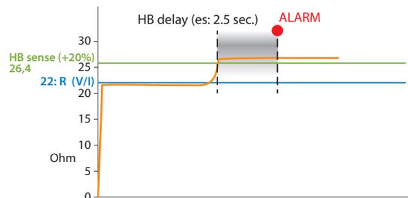
Sensitivity (HB sense) and delay (HB delay) can be varied according to the application (see parameters on pages 32-33).
