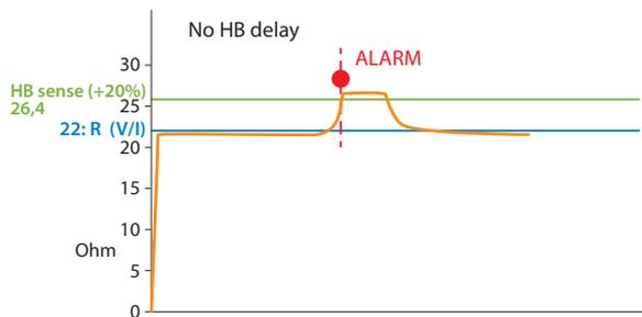
Using the HB Delay parameter, the alarm intervention can be delayed.
