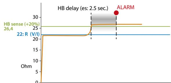
Sensitivity (HB sense) and delay (HB delay) can be varied according to the application (see parameters on pages 32).
