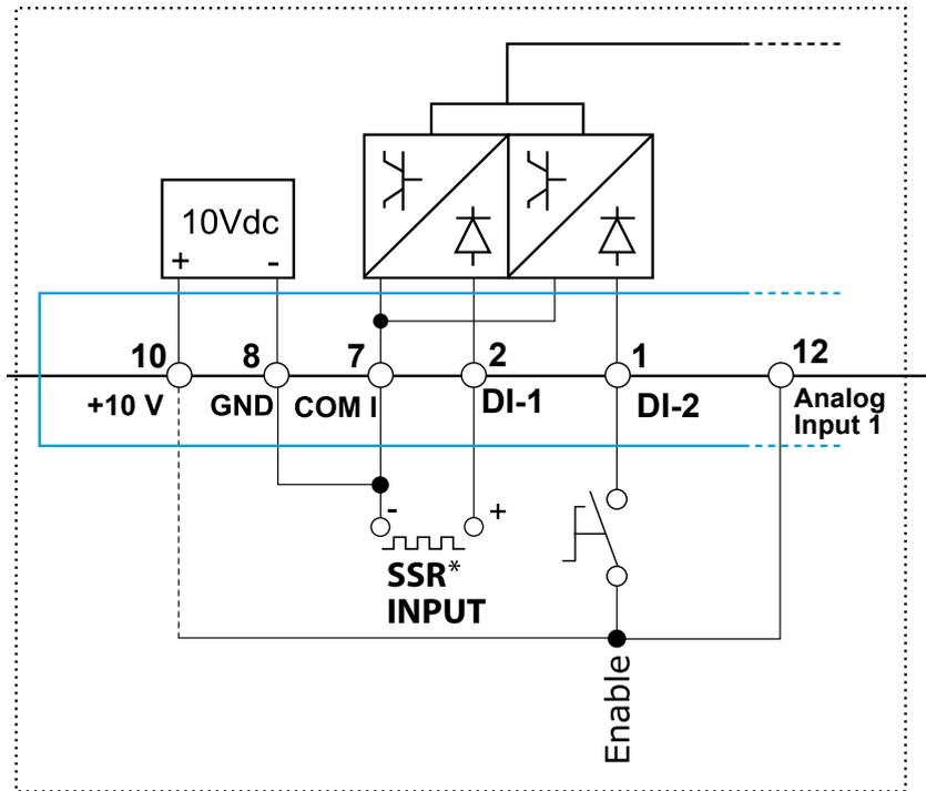
\* SSR Input: 4 ÷ 30Vdc 5mA Max (ON ≥4Vdc OFF <1Vdc)
