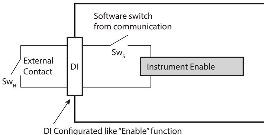
$Sw_H$  = Switch hardware       $Sw_S$  = Switch software
